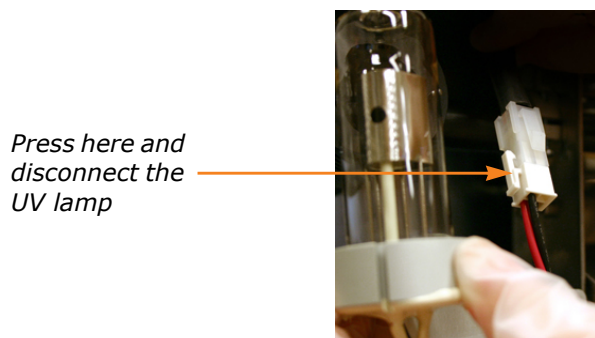
Figure 5-14. Disconnect the UV Lamp
