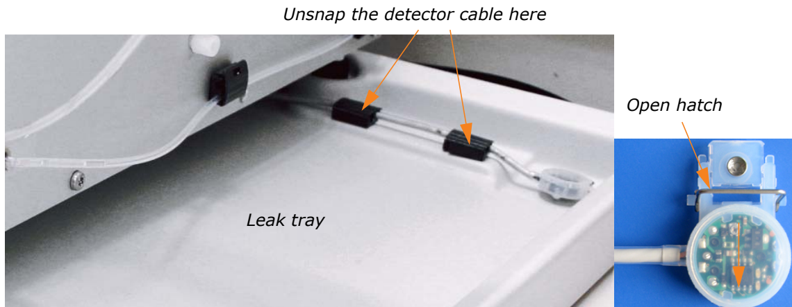
Figure 5-5. Isolera System with Leak Detector
