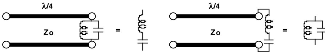
The quarter wave sections transform the center shunt parallel resonant circuit admittance to a series impedance that is a series resonant circuit.
