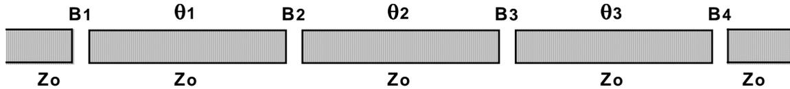
It can be seen that the equivalent circuit can incorporate the short admittance inverter, and that the resonators can be shortened to incorporate the negative lengths required. This filter can be designed by reference to a lumped element prototype, using the equivalent circuits of the near-half-wave resonators and identifying corresponding parameters.
