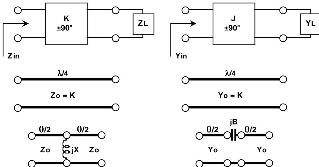
For the impedance inverter,  $Z_{in} = K^2/Z_L$
