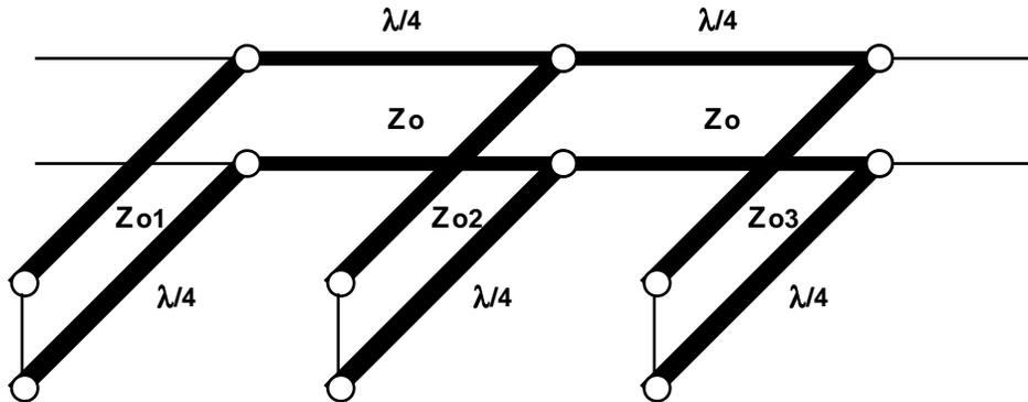
This filter can also be configured as a bandstop filter by using open rather than shorted stubs. While it's easy to see that this filter will pass the center frequency for which the lines are all  $\lambda/4$ , we would like to be able to design such a filter using lumped element prototypes.
