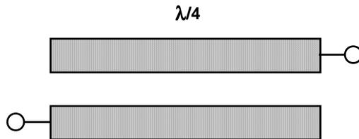
The equivalent circuit of two coupled  $\lambda/4$  open lines can be shown to be as depicted here:
