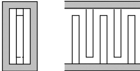
The interdigital filter structure typically takes the form shown here, with the casing and fingers typically silver plated machined aluminum; another form uses cylindrical pins pressed into a housing, but there can be problems with the joint at the high current end of the transmission line fingers:
