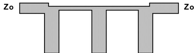
Although the lumped element filter has only lowpass response, the periodic nature of distributed elements results in harmonic responses because of the periodic nature of the structure. In this case, there are responses centered on  $4nf_c$ , where  $n$  can take any positive integral value. This is a general characteristic of distributed-element filters, and can be a problem if unanticipated in system designs.
