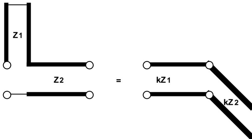
This diagram shows the equivalence for the most commonly used identity, which removes a series stub by transforming it to a shunt stub along with adjustment of characteristic impedances of the  $\lambda/8$  lines.
