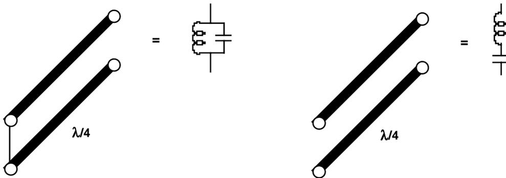
But it is important to note that a parallel tuned circuit is transformed through a  $\lambda/4$  line to the impedance of a series tuned circuit, and vice versa. This allows us to determine the equivalent circuit of the transmission line filter.
