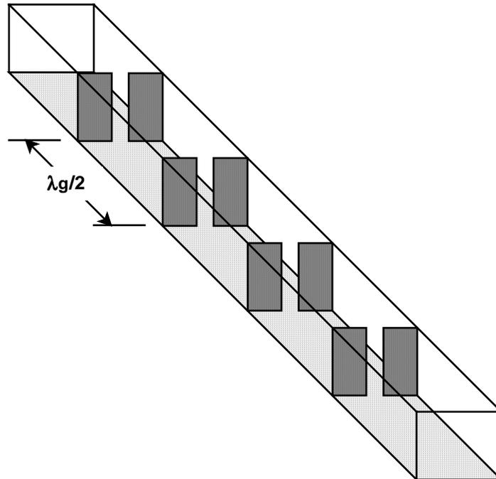
Waveguide filters generally employ iris-coupled resonant sections in a pattern similar to the capacitive coupled resonator filter. The waveguide can be cut with a saw and the iris material soldered in before plating. As with other metallic filters, it is not unusual for a designer to take advantage of the opportunity to have tuning screws to accommodate small tolerance variations in the filter.
