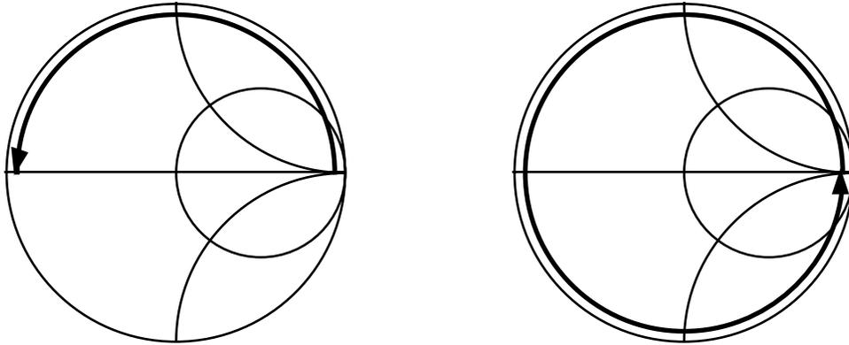
When we tune the last resonator, we see the load at the output of the filter. But we can still get the proper tuning by observing the additional  $90^\circ$  phase change.
