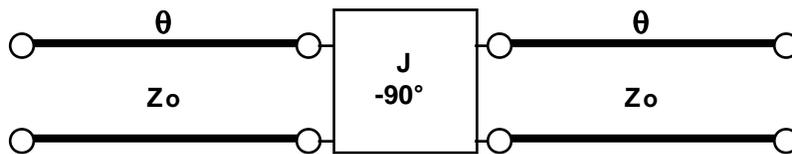
So we can see that a structure of a number of coupled lines will admit to an equivalent circuit of alternating series and parallel resonant circuits, and the design parameters of the prototype filter can be imposed onto the structure of parallel coupled lines.
