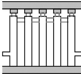
One major benefit of the combline filter is that, uniquely among the forms shown above, it can be designed so that the interplay of distributed and lumped elements can be used to eliminate the higher order passbands. As we will see in later lectures, this is a very significant advantage for large-signal circuits that have substantial harmonic energy.
