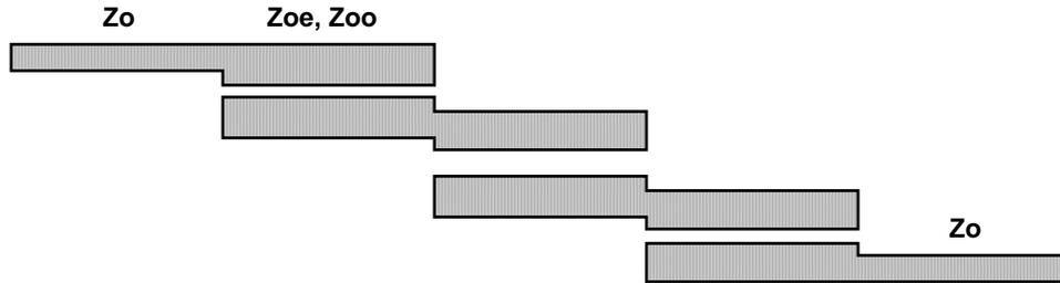
In microstrip or stripline, the transmission line conductors of the coupled line filter take the form shown here, with the offsets between connected  $\lambda/4$  sections added to permit seeing the individual coupled line pairs.
