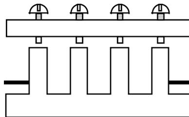
Consider a filter such as a comb-line filter which has been designed but must now be tuned. If all the tuning screws are shorted to their respective resonators, the output admittance at, say, the input port plane is very high. As that resonator is tuned, the reflection coefficient stays high because the rest of the filter is still shorted, but the phase of the reflection coefficient can range through a  $180^\circ$  range. If we stop at  $90^\circ$  phase
