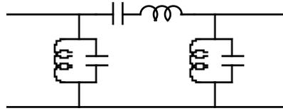
Thus, the equivalent circuit of the bandpass filter using quarter wave lines is the same as the prototype lumped element filter that is created through the customary transformation from lowpass to bandpass prototype filters. Using the known relationships between transmission line  $Z_0$  and the L and C of the equivalent resonance, we can identify the relationships between the required L and C of the prototype circuit and the  $Z_0$  we need for the shunt stubs.
