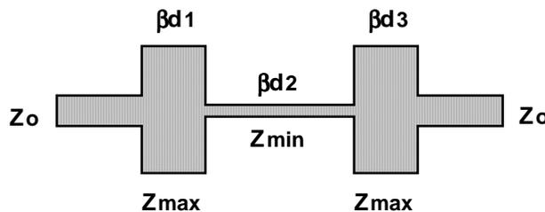
As a worked example, consider the design of a maximally flat three-section lowpass filter that has a cutoff frequency of  $f_c = 1$  GHz. The highest practical impedance is  $Z_{max} = 120$  ohms and the lowest practical impedance is  $Z_{min} = 12$  ohms. Assume we have
