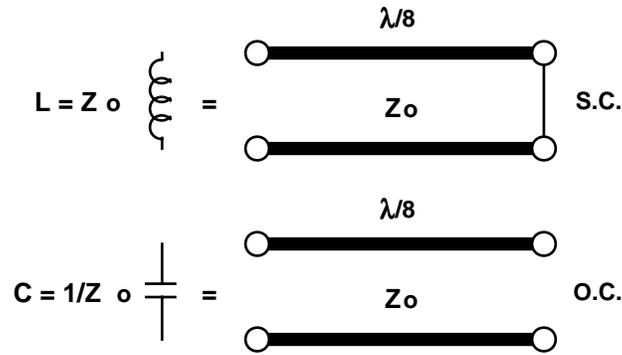
The  $\lambda/8$  transmission line sections are called commensurate lines, since they are all the same length in a given filter.
