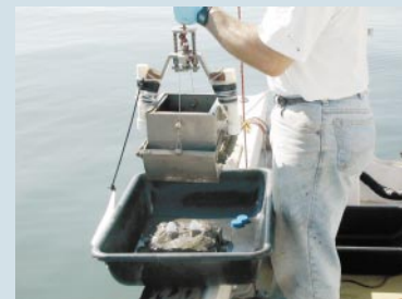
Sediments were collected using a .038 m2 Birge-Eckman stainless steel box core
