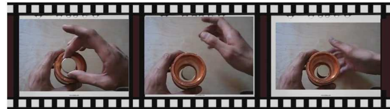
FIGURE 1: Check out the video on Youtube! Use the search terms, "neodymium magnet copper pipe". The magnet seems to take forever traversing the pipe. Very cool
