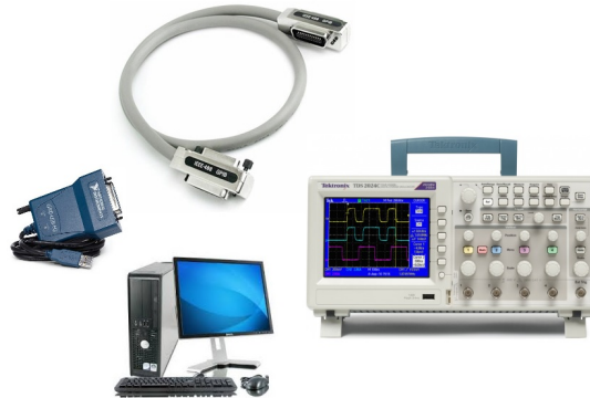
Figure 8: Instruments such as the DSO can acquire data using the signal processing present in the instrument itself, and be controlled by LabView software via the pc through the gpib bus, using the hardware shown above. Gpib cabling is generally required.
