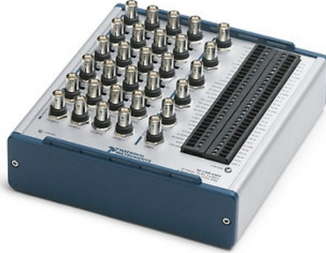
Figure 4: The NI USB-6343 has 4 analog outputs and 23 analog inputs, with a maximum digitization rate of 500ks/s.
