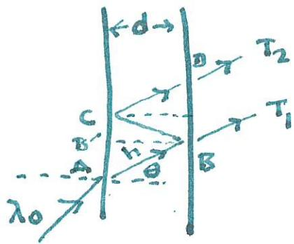
One sees the formula for the accumulated phase shift between successive (adjacent) transmitted rays through a planar Fabry-Perot etalon
