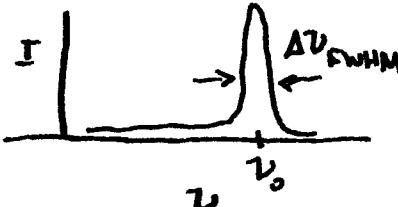
An ensemble of atoms in thermal equilibrium at temp T produces a 'Doppler-Broadened' line where the Full WIDTH-HALF MAX (FWHM) is determined by T,  $\Delta\nu_D = \nu_0 \sqrt{\frac{8kT\ln 2}{mc^2}}$  ...†
