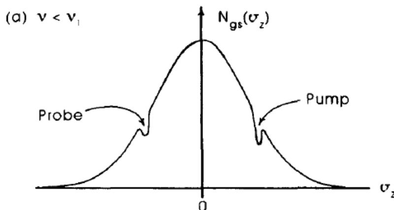
tral lines. To understand these it helps to look at Fig. 4, which shows the number of atoms in the ground state,  $N_{gs}(v_z)$  as a function of atomic velocity  $v_z$  (where positive  $v_z$  is parallel to the probe beams). In Fig. 4(a) the laser
