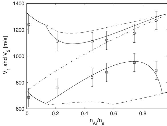
FIG. 6. Comparison of data and the prediction of the revised theory. The circles are the measured argon drift velocity and the squares are the measured xenon drift velocity. The solid line is the new prediction while the dashed line is the old prediction. The system Bohm velocity is represented by the dashed dotted line.
