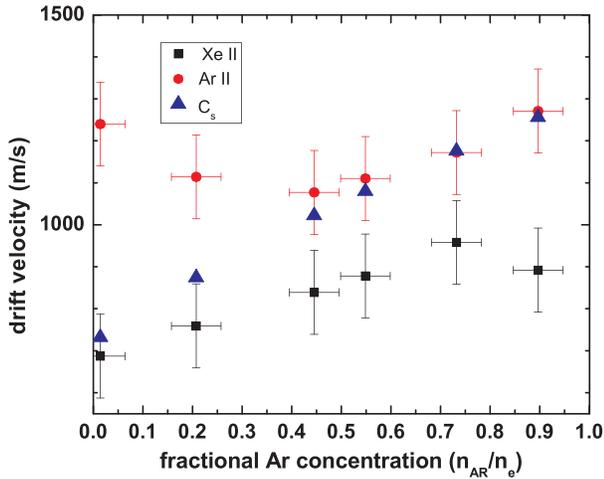
FIG. 2 (color online). Measured drift velocities and system sound velocities with respect to the argon ion concentration ratio.
