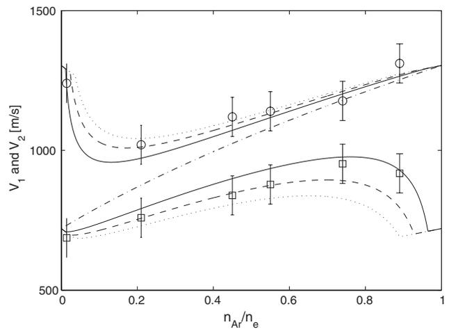
FIG. 5. Circles and squares are the measured argon and xenon velocities, respectively. Lines are prediction curves with ion temperatures of 0.005 eV (solid), 0.01 eV (dashed) and 0.015 eV (dotted). The solid line in the middle is the system sound velocity.
