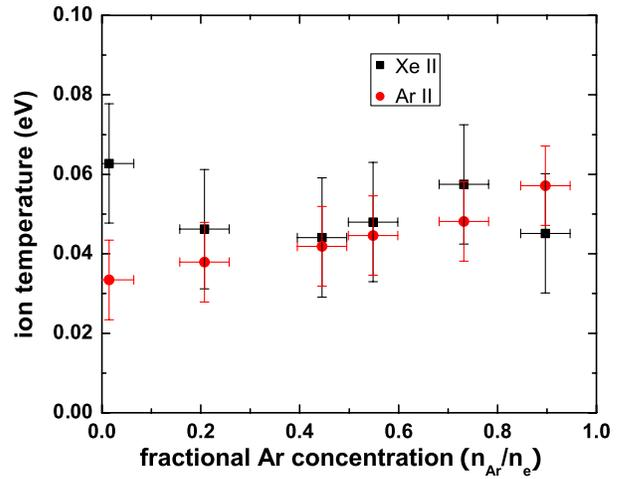
FIG. 4 (color online). Ion temperature graphed versus argon ion concentration.
