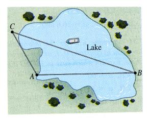
2. To estimate the length CB of the lake in the figure that follows, a surveyor measures AB and AC to 89m and 75m, respectively, and  $\angle CAB$  to be 95°. Find the approximate length of the lake.
