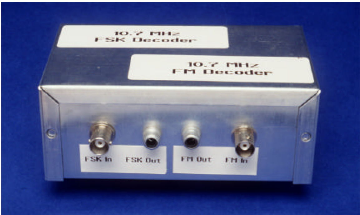
Fig. 10b. Front panel of IF amplifier/decoder box.
