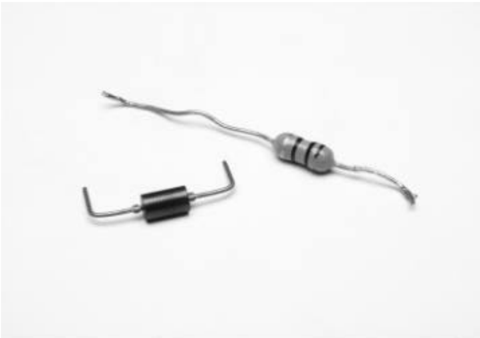
Fig. 3b. RF chokes (RFCs) can employ ferrite beads (left) or molded inductors (right).
