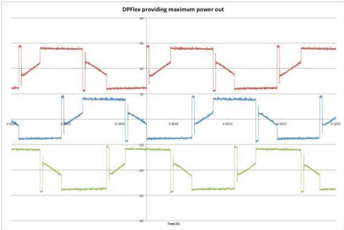
Figure 159. Voltage across all three motor phases at full power.
