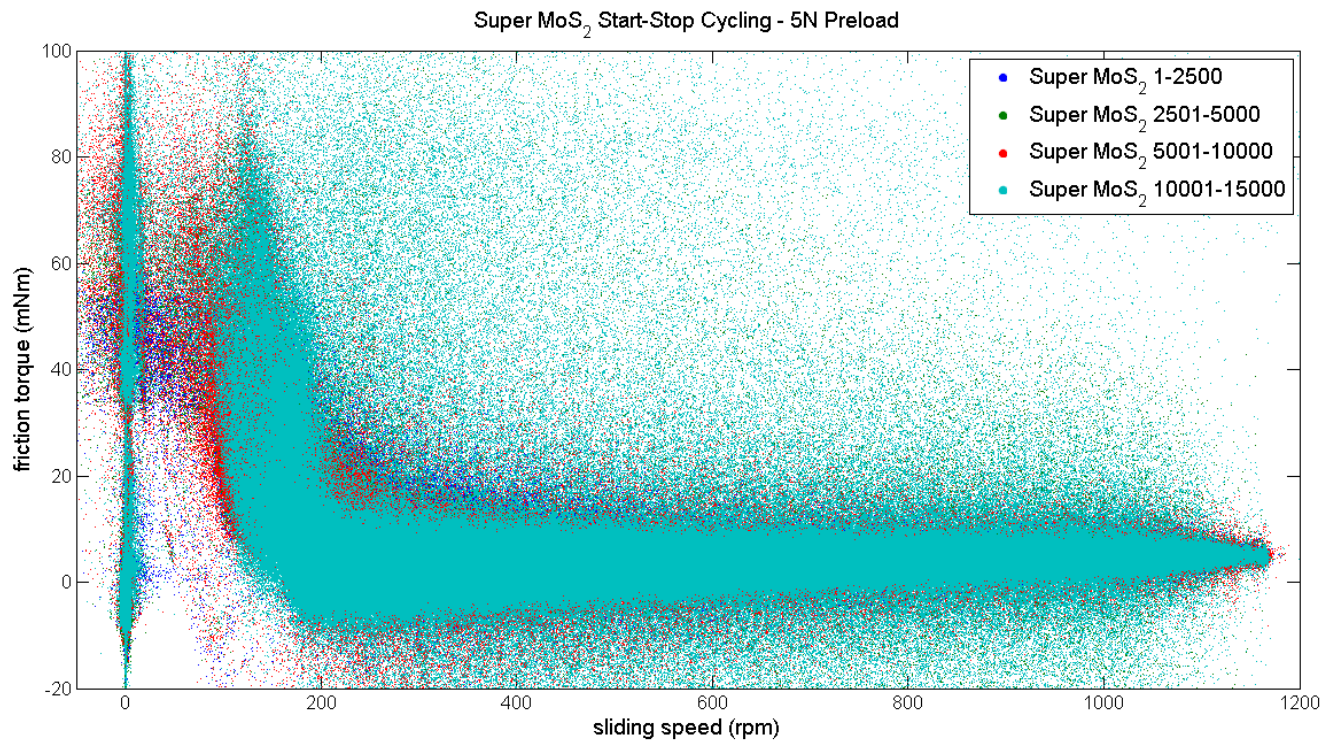
Figure 156: Friction torque data for Super MoS 2 during cycle testing.
