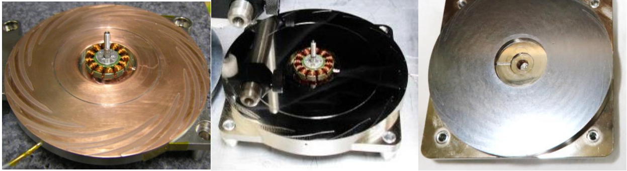
Figure 11. Three spiral groove air bearing designs: V4 (left), V5 (middle), and final (right).
