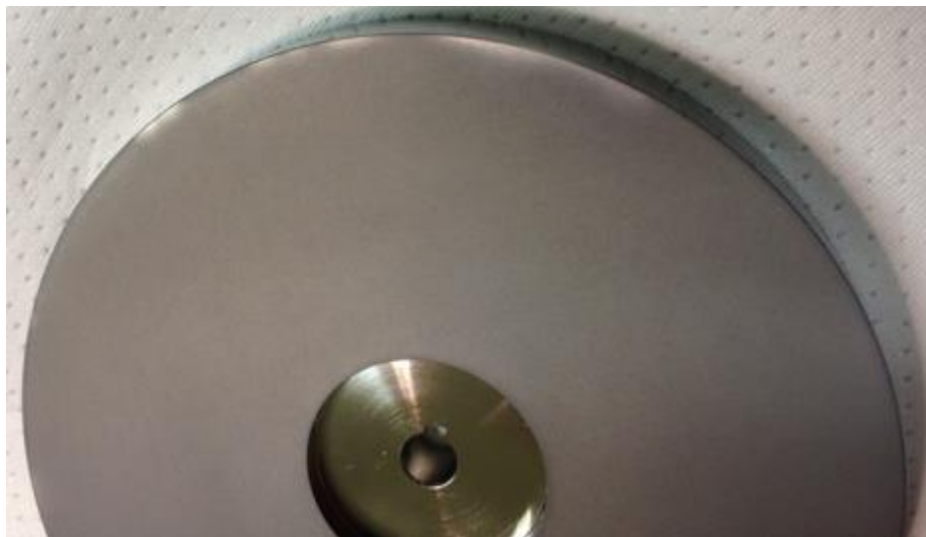
Figure 140. Impeller substitute coated with low energy deposition i-Kote, prior to installation.
