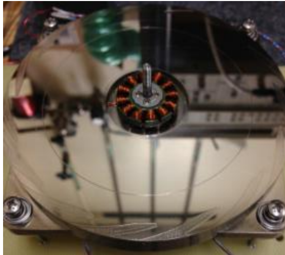
Figure 157. Motor stator mounted on baseplate.
