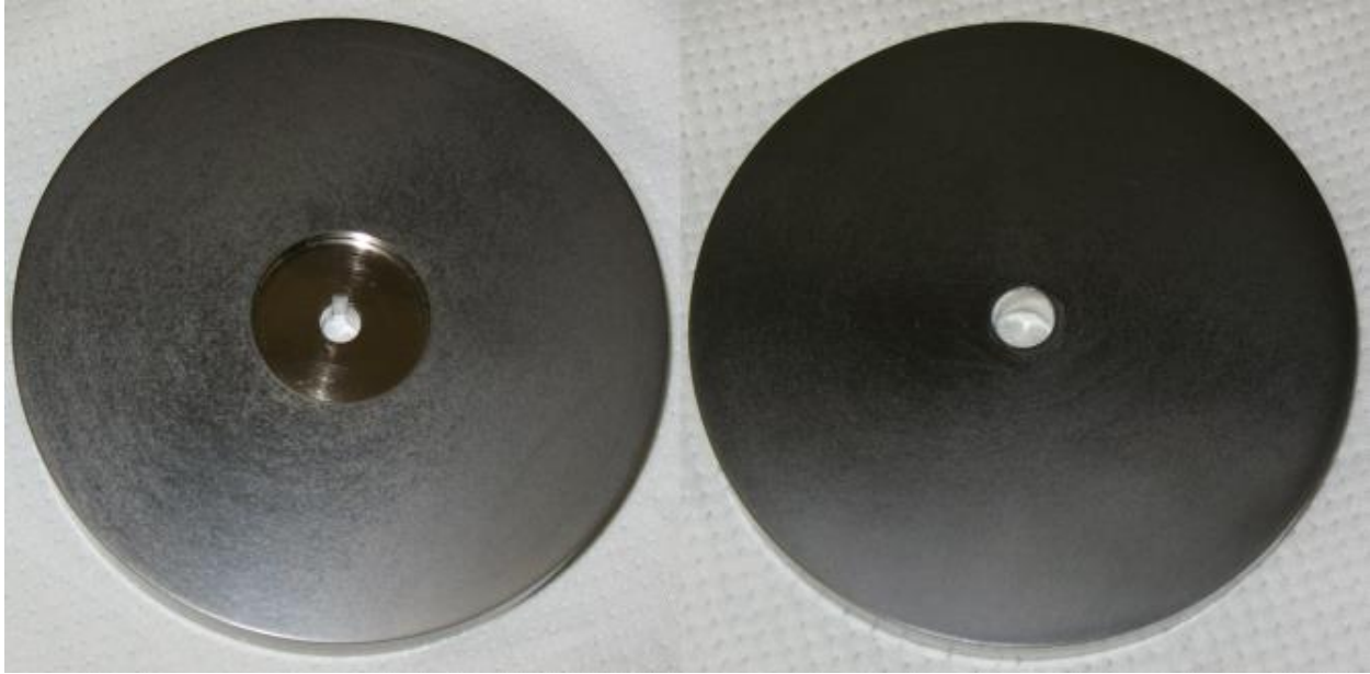
Figure 144: Parts coated using standard deposition, prior to installation.
