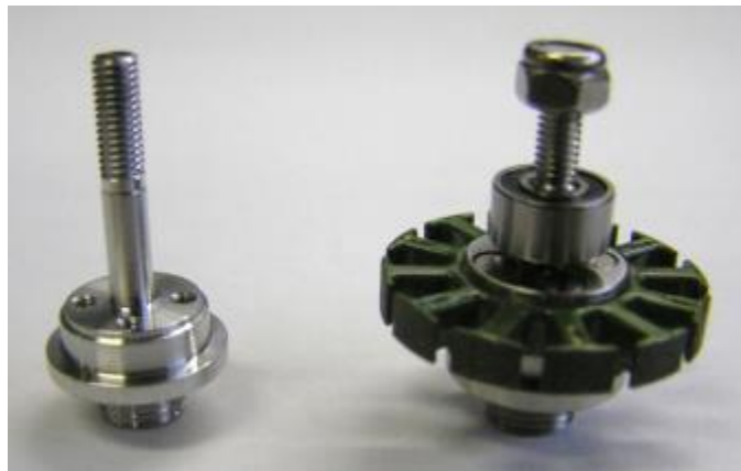
Figure 116. New motor stator mount and shaft.
