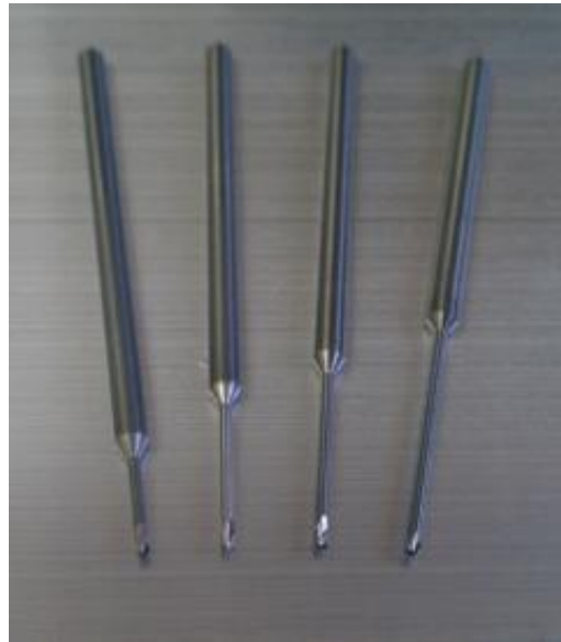
Figure 33. Progressively higher aspect ratio tools were used to machine the V5 impeller.
