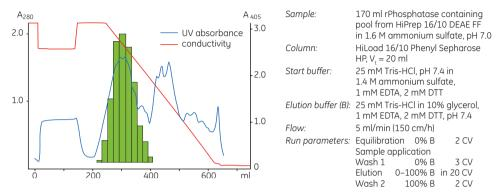
**Fig 9.8.** Intermediate purification step using hydrophobic interaction. The phosphatase activity is represented by the green bars (absorbance at 405 nm).
