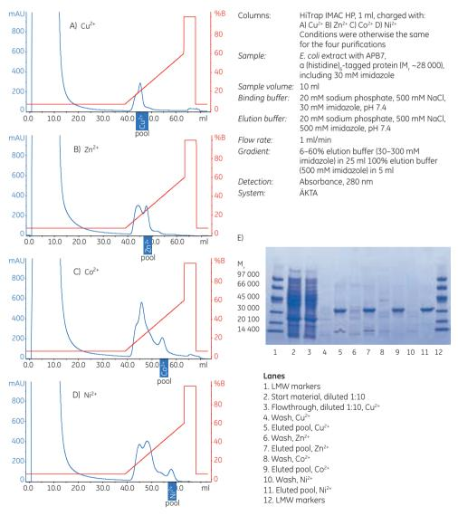
**Fig 4.4.** Purification of APB7, a (histidine)<sub>6</sub>-tagged protein expressed in *E. coli* BL-21 on four different HiTrap IMAC HP 1 ml columns charged separately with metal ions. (A) Cu²+, (B) Zn²+, (C) Co²+, or (D) Ni²+. Pools selected after SDS-PAGE of individual 1 ml fractions (not shown) are indicated. (E) SDS-PAGE analysis: reducing conditions on ExcelGel SDS Gradient 8–18; Coomassie staining.
