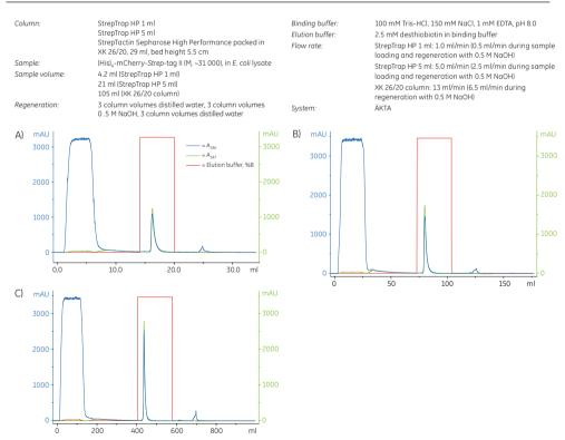
**Fig 7.5.** Scaling up the purification of  $(His)_c$ -mCherry-Strep-tag II, (A) StrepTrap HP 1 ml, (B) StrepTrap HP 5 ml, (C) StrepTactin Sepharose High Performance XK 26/20 with 5.5 ml bed height, 29 ml.
