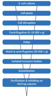
**Fig 10.1.** General scheme for the extraction, solubilization, and refolding of (histidine)<sub>6</sub>-tagged proteins produced as inclusion bodies in *E. coli* cells.
