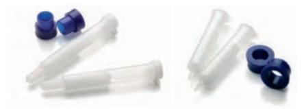
Fig 11.6. PD MiniTrap G-25 prepacked columns for cleanup of proteins with  $M_r > 5000$  in sample volumes up to 500  $\mu$ l (PD MiniTrap G-25; left) and 1.0 ml (PD MidiTrap G-25; right).
