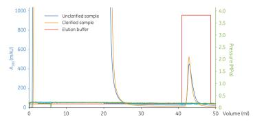
**Fig 3.44.** Comparison study loading unclarified (blue line) and clarified (orange line) *E. coli* samples containing the histidine-tagged protein GEHC1-(His), on HiTrap TALON crude. Overlay of absorbance curves.
