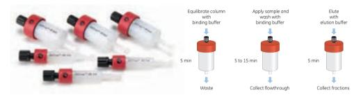
**Fig 5.8.** GSTrap HP, GSTrap 4B, and GSTrap FF 1 ml and 5 ml columns allow convenient and simple one-step purification of GST-tagged proteins. Simple purification of GST-tagged proteins is shown at right.
