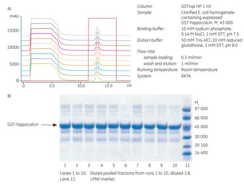
**Fig 5.9.** (A) Confirmation of the stability of Glutathione Sepharose High Performance prepacked in 1 ml GSTrap HP columns. Chromatographic overlay of 10 repetitive purifications. (B) Coomassie-stained nonreduced SDS-polyacrylamide gel (ExcelGel SDS Gradient 8–18) of pooled fractions from repetitive purification runs shown in (A).
