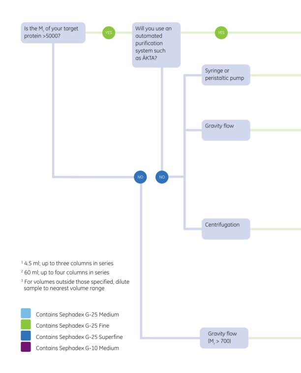
Fig 11.1. Selection guide: Prepacked columns for desalting/buffer exchange.
