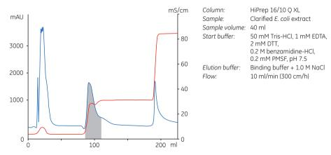
Fig 9.4. Capture using IEX. The elution position of DAOCS is shaded.
