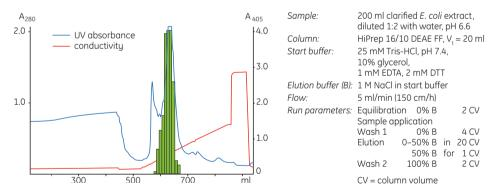
**Fig 9.7.** Capture step using IEX. The phosphatase activity is represented by the green bars (absorbance at 405 nm).
