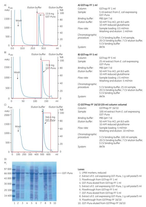
**Fig 5.16.** Purification and scale-up of GST-Pur $\alpha$  on (A) GSTrap FF 1 ml, (B) GSTrap FF 5 ml, and (C) GSTPrep FF 16/10. (D) SDS-PAGE analysis of GST-Pur $\alpha$  on ExcelGel Homogeneous 12.5% using Multiphor II followed by Coomassie staining. Due to the slow binding kinetics of GST, some of the applied protein was found in the flowthrough.
