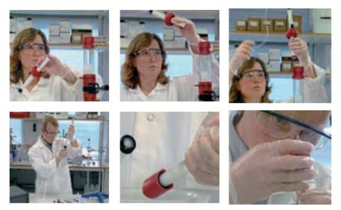
Fig A6.1. "Column Packing — The Movie" provides a step-by-step demonstration of column packing.
