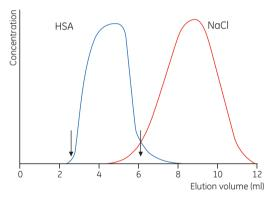
Fig 11.8. Removal of NaCl from albumin solution. A PD-10 Desalting column was equilibrated with distilled water. A total of 23.8 mg of albumin was recovered in 3.5 ml of eluent corresponding to a yield of 95.3% (between arrows).
