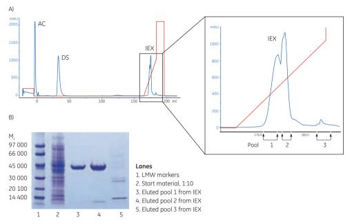
**Fig 4.6.** (A) AC-DS-IEX with an enlargement of the IEX peaks and the collected pools to the right. Yield: 9.4 mg in pools 1 + 2. (B) SDS-PAGE of eluted pools from IEX. The gel was stained with Coomassie.
