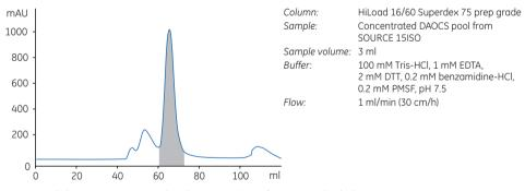
Fig 9.6. Polishing step using GF. The elution position of DAOCS is shaded.
