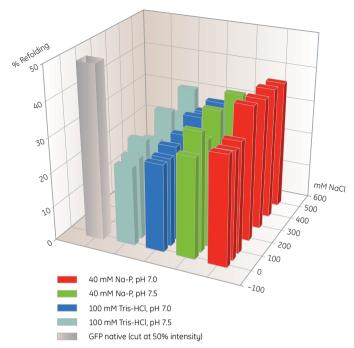
**Fig. 10.4.** Screening of IMAC refolding conditions for histidine-tagged GFP using His MultiTrap FF. This initial screen covered buffer substances, pH and salt concentrations. Data kindly provided by J. Buchner, M. Haslbeck and T. Dashivets, Munich Technical University, Germany.
