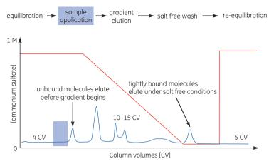
Fig A11.5. Typical HIC gradient elution. Blue line = absorbance; red line = conductivity (salt concentration).
