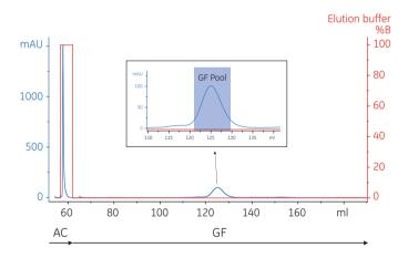
**Fig 6.3.** Automated purification of MBP2\*-paramyosin-δ-Sal using the two-step AC-GF protocol on MBPTrap HP 1 ml (AC) and HiLoad 16/60 Superdex 200 pg (GF).
