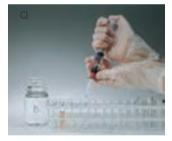
**Fig 5.10.** Using a GSTrap column with a syringe. A) Prepare buffers and sample. Remove the column's top cap and snap off the end. B) Load the sample and begin collecting fractions. C) Wash and elute, continuing to collect fractions.
