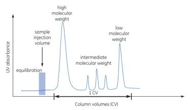
Fig A11.7. Typical GF elution.
