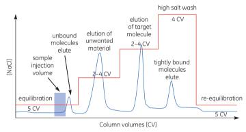
Fig A11.4. Step elution. Blue line = absorbance; red line = conductivity (salt concentration).
