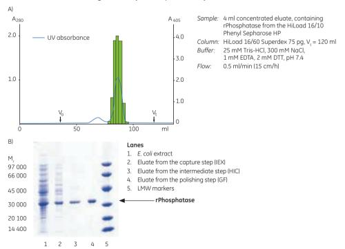
**Fig 9.9.**(A) Polishing step using GF. The phosphatase activity is represented by the green bars (absorbance at 405 nm). (B) Purity check by SDS-PAGE. The proteins were stained with Coomassie Brilliant Blue.
