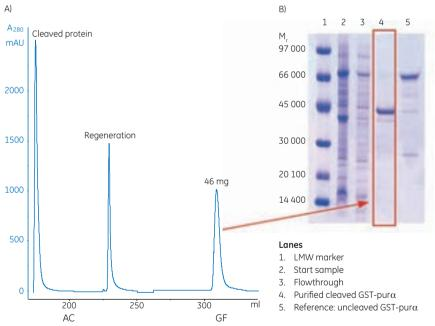
**Fig 5.22.** (A) Two-step protocol for automatic GST-tagged protein cleavage with PreScission Protease and purification. (B) Analysis by SDS-polyacrylamide gel (Coomassie staining) of the untagged target protein after purification and cleavage.
