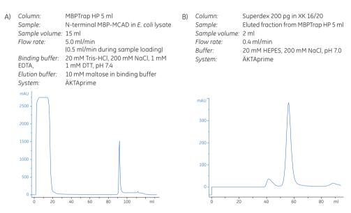
Fig 6.5. Purification of MCAD on (A) MBPTrap HP followed by (B) Superdex 200 pg.
