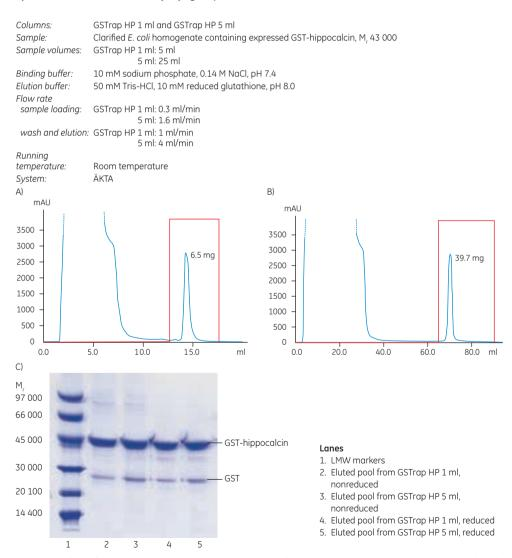
**Fig 5.11.** Scale-up from (A) GSTrap HP 1 ml to (B) GSTrap HP 5 ml. (C) Coomassie-stained reduced and nonreduced SDS-polyacrylamide gel (ExcelGel SDS Gradient 8–18) of fractions from purification shown in Fig 5.11A–B.
