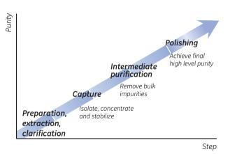
Fig 9.1. Preparation and CIPP (Capture - Intermediate Purification - Polishing).
