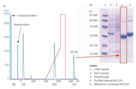
**Fig 3.53.** (A) Four-step protocol for purification of (histidine)<sub>c</sub>-tagged protein cleaved with AcTEV protease. (B) SDS-PAGE analysis. The gel was stained with Coomassie.
