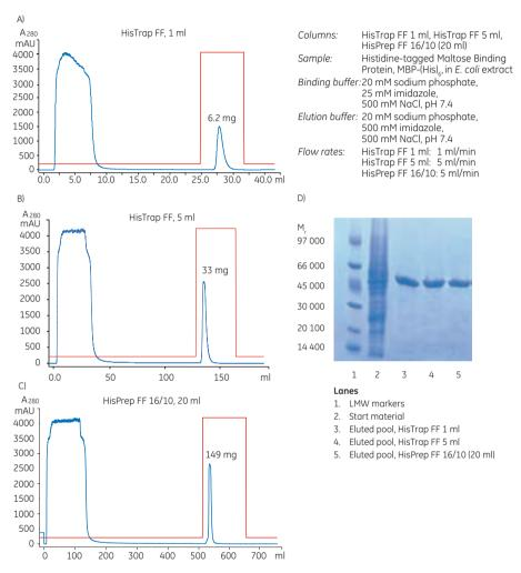
Fig 3.13. Scale-up from (A) HisTrap FF 1 ml via (B) HisTrap FF 5 ml to (C) HisPrep 16/10 (20 ml) prepacked column. The samples loaded contained approximately 8, 40, and 160 mg of MBP-(His) $_{\rm c}$ , respectively. Recovery in milligrams is shown in each chromatogram. (D) SDS-PAGE (ExcelGel SDS Gradient 8–18) under nonreducing conditions confirms that scaling up from the 1 ml to the 20 ml column does not significantly affect the purification result.
