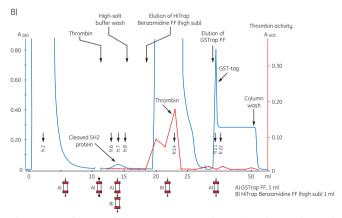
**Fig 5.23.** Purification of GST-SH2 GST-tagged protein with on-column cleavage and post-cleavage removal of thrombin using GSTrap FF and HiTrap Benzamidine FF (high sub) columns. (A) SDS-PAGE analysis of various sample processing steps. ExcelGel SDS Gradient 8–18%, Coomassie blue staining. (B) Chromatogram (blue: absorbance at 280 nm) and thrombin activity curve (red) demonstrating all steps in the purification of the SH2 domain.
