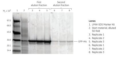
Fig 3.43. SDS-PAGE analysis of elution fractions from a purification of GFP-His (M. 28 000) added to E. coli lysate. The SDS-polyacrylamide gel (reducing conditions) was stained with Deep Purple Total Protein Stain and analyzed with ImageOuant TL software. The experiment was performed in triplicate. The first elution fraction contained 96% of the purified protein.
