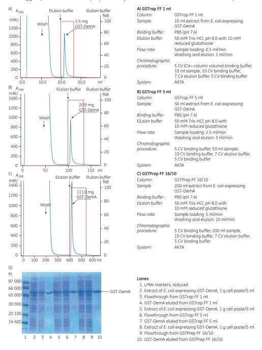
Fig 5.15. Purification and scale-up of GST-DemA on (A) GSTrap FF 1 ml, (B) GSTrap FF 5 ml, and (C) GSTPrep FF 16/10. (D) SDS-PAGE analysis of GST-DemA on ExcelGel Homogeneous 12.5% using Multiphor™ II followed by Coomassie staining. Due to the relatively slow binding kinetics of GST and rather high load, some of the applied protein was found in the flowthrough.
