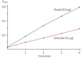
Fig 5.19. Typical results of a CDNB assay for GST-tagged proteins. 53 µg of total protein from an E. coli TG1/pGEX-4T-Luc sonicate and 0.8 µg of total protein eluted from Glutathione Sepharose were assayed according to instructions included with the GST Detection Module.
