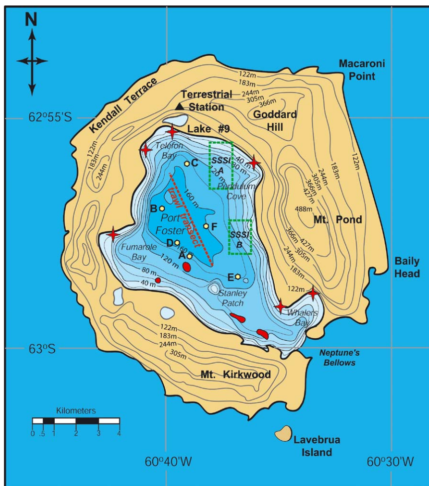
Fig. 2. Chart of Deception Island with corrected bathymetry of Port Foster and showing, fumaroles = \star (Cooper et al., 1998), submarine volcanic domes = \bullet (Rey et al., 1995) SSSI sites (A and B), long-term mooring locations (A—thermistor array, B—thermistor array with acoustic Doppler current profiler, C—thermistor array, D—sediment traps and time-lapse camera, E—vertically profiling acoustic array, F—vertically profiling pump sampler), pelagic and benthic trawling transect, and the Terrestrial station ( \blacktriangle ).
